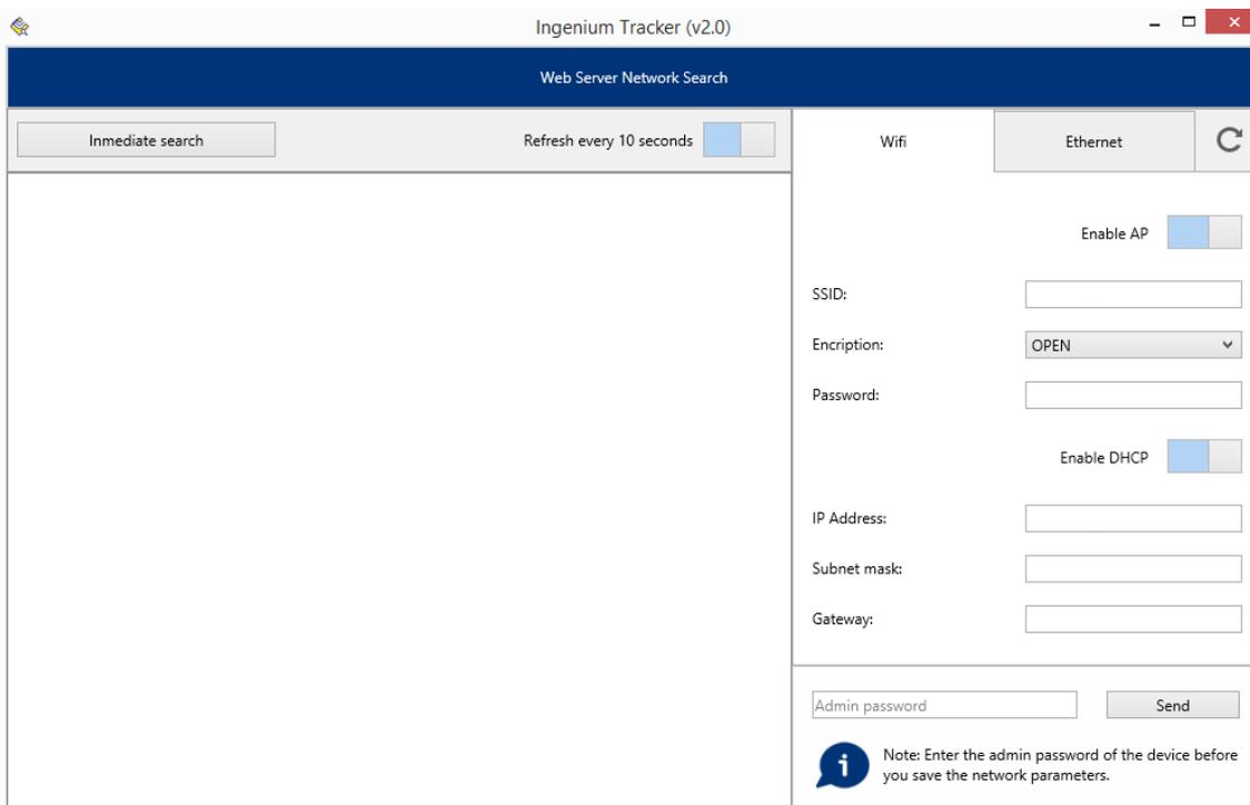
Using the software Ingenium Tracker is a preliminary step for the subsequent programming of the project on the web server or the touch screens from the SiDE KNX software.
