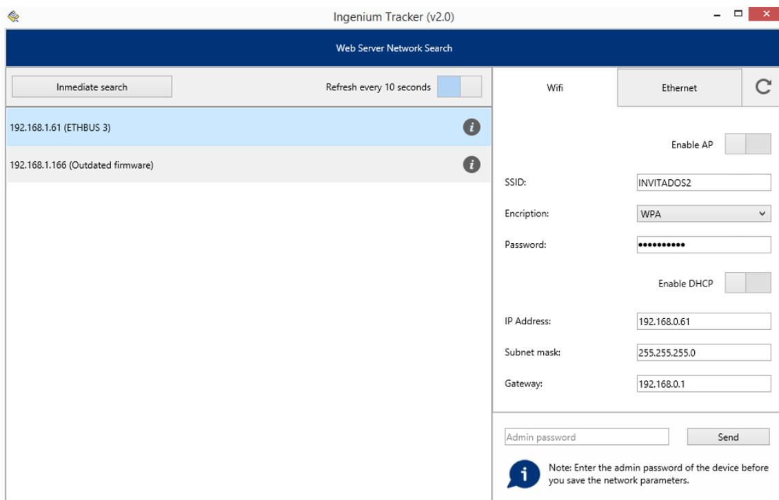
Once found the device can be selected in the list and accessed with a click for its configuration. The list of found devices can be deleted at any time by clicking the right mouse button and clicking *clear list*.
