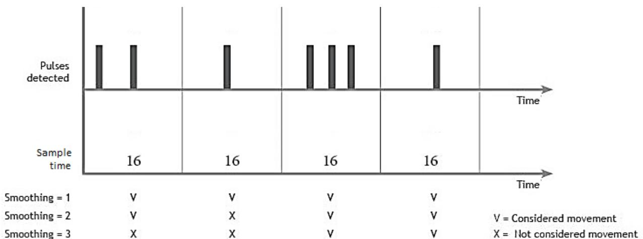
Any movement that generates a number of pulses higher than the **smoothing**, within a given sampling time, is considered a "motion detection" by the sensor. For the same sampling time, increasing the smoothing means that the movement should be faster and higher to generate a "motion detection" because more pulses are necessary.
