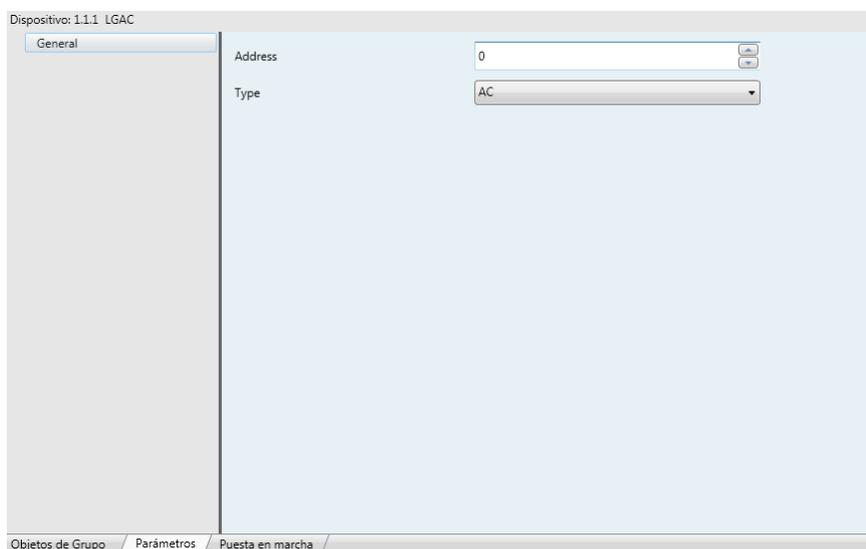
The programmer must add as much as LGAC-KNX virtual devices to the ETS project as LG AC indoor units there are modifying the address parameter in each one.
